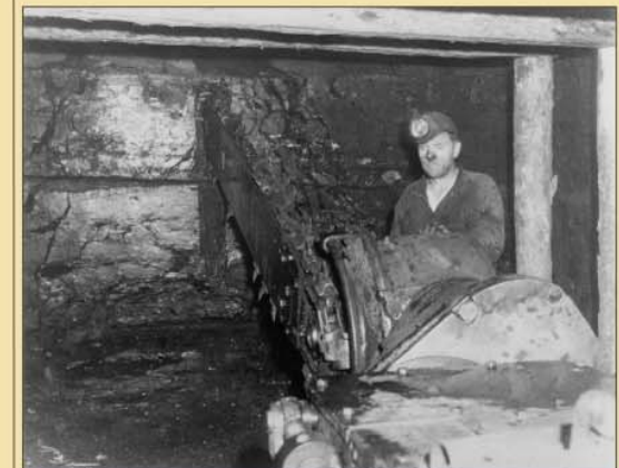
Universal Coal Cutter. A coal cutter was being repaired in the room where the explosion took place.
